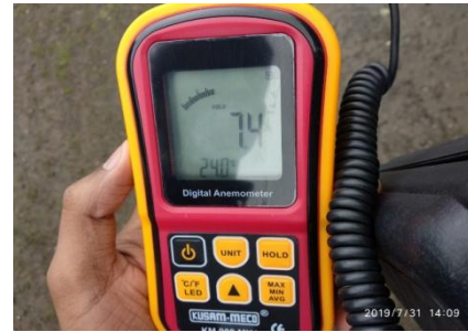
Fig.5. Velocity measurement using Anemometer
